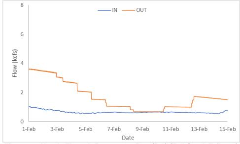
Figure 64. Hourly Flows Inflow vs. Outflow (RO) (Fall Creek Tailrace)
