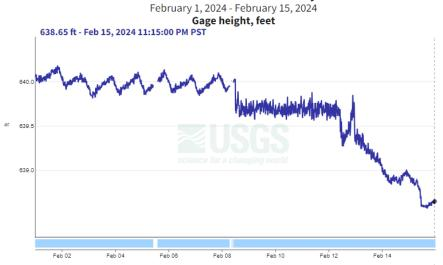
Figure 67. Gauge Height (feet); below Dexter Dam, Middle Fork Willamette.
