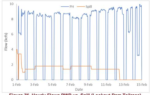
Figure 76. Hourly Flows PWR vs. Spill (Lookout Dam Tailrace).
