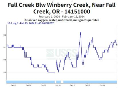
Figure 62. Dissolved Oxygen (mg/L), Fall Creek below Winberry Creek, Near fall Creek, OR
