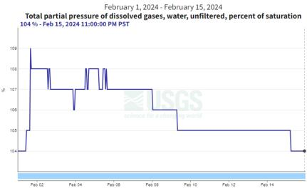
Figure 47. Total Dissolved Gas Saturation (%); below Cougar Dam, South Fork McKenzie River.
