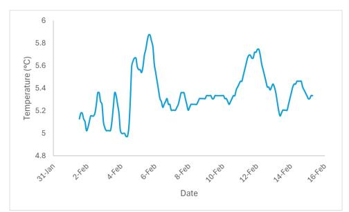
Figure 24. Temperature at RST (Big Cliff Dam).
