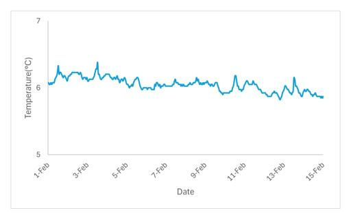
Figure 49. Temperature at PWR RST (Cougar Dam).
