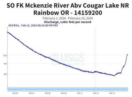
Figure 53. Discharge (cfs); South Fork McKenzie above Cougar Dam.
