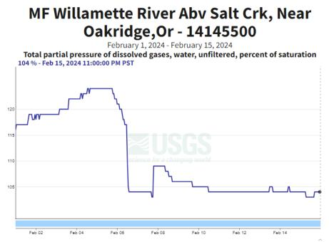
Figure 89. Total Dissolved Gas Saturation (%); below Hills Creek Dam – Middle Fork Willamette River.
